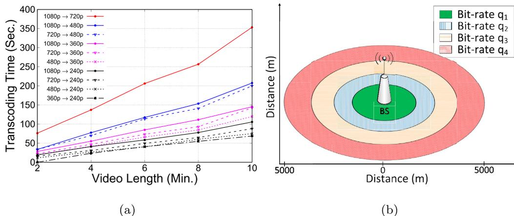
**Fig. 1.** (a) Time taken to transcode videos of different playtime from a higher bit-rate input video to a lower bit-rate video. (b) Supportable video bit-rate ( $q_1 > q_2 > q_3 > q_4$ ) based on the UE distance from the cellular Base Station (BS).
