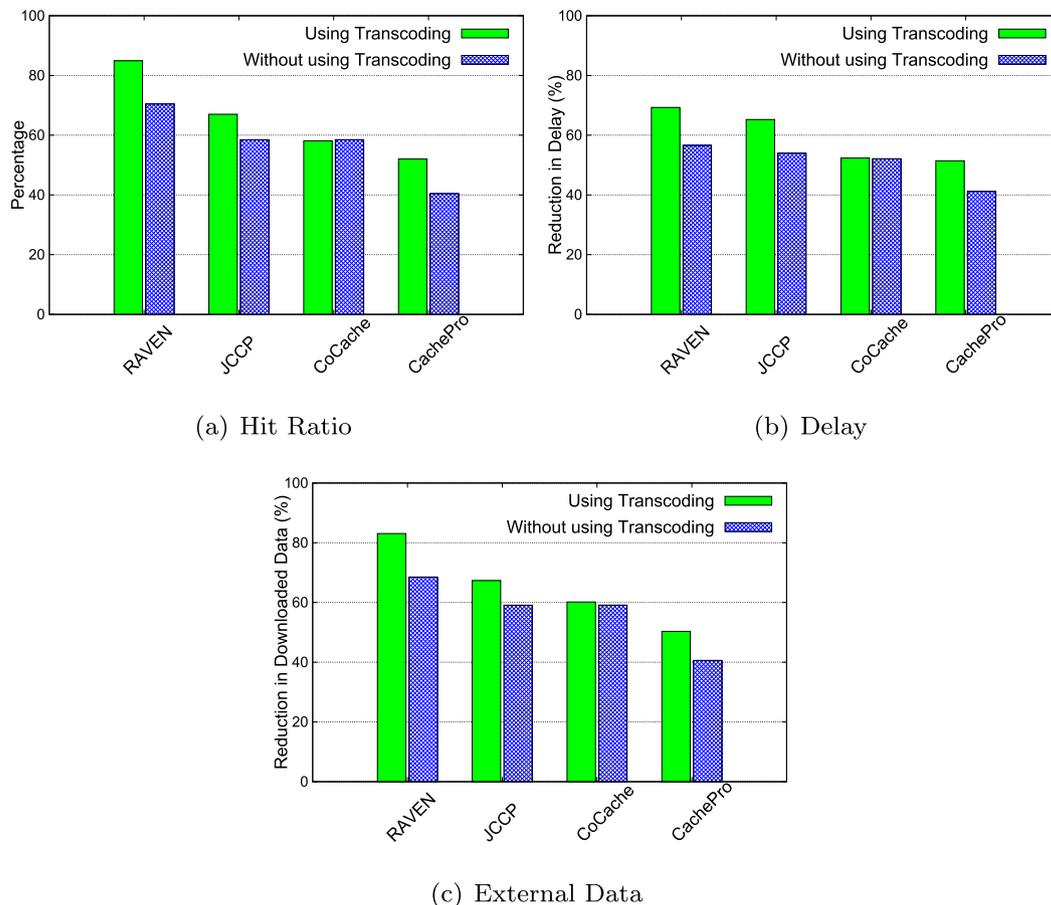
Fig. 8. Effect of the use of transcoding on hit-rate, reduction in delay, and downloaded data.
