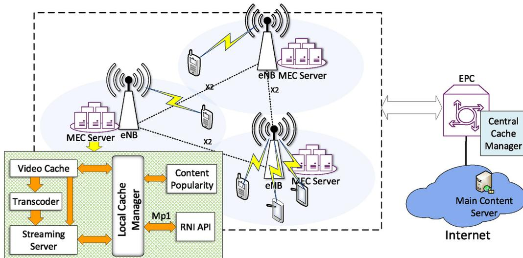
Fig. 2. MEC video caching system architecture.
