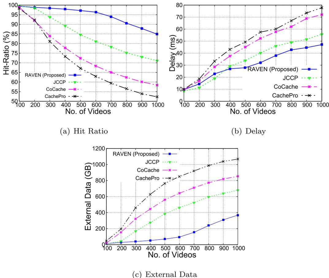
Fig. 7. Effect of change in number of videos in library on hit-rate, reduction in delay, and downloaded data.
