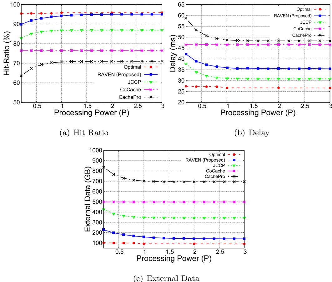
Fig. 5. Change in (a) hit ratio, (b) delay, and (c) external data with increase in processing power.
