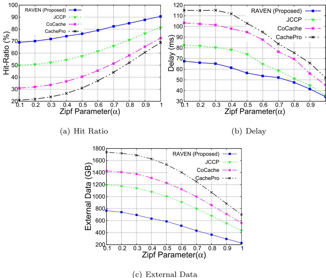
Fig. 6. Change in hit ratio, delay, and external data with change in skewness of video popularity distribution.
