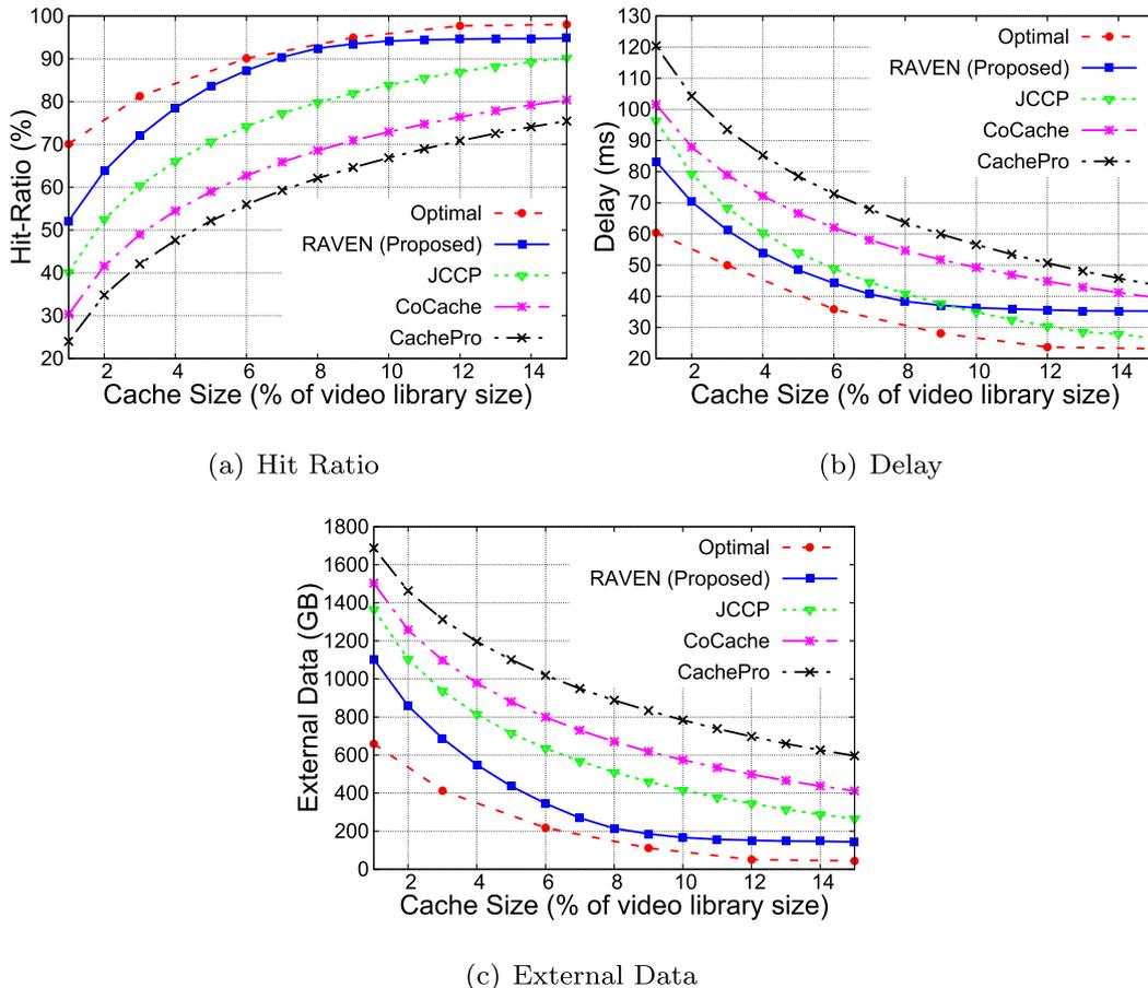
Fig. 4. Change in hit ratio, delay, and external data with increase in cache size.
