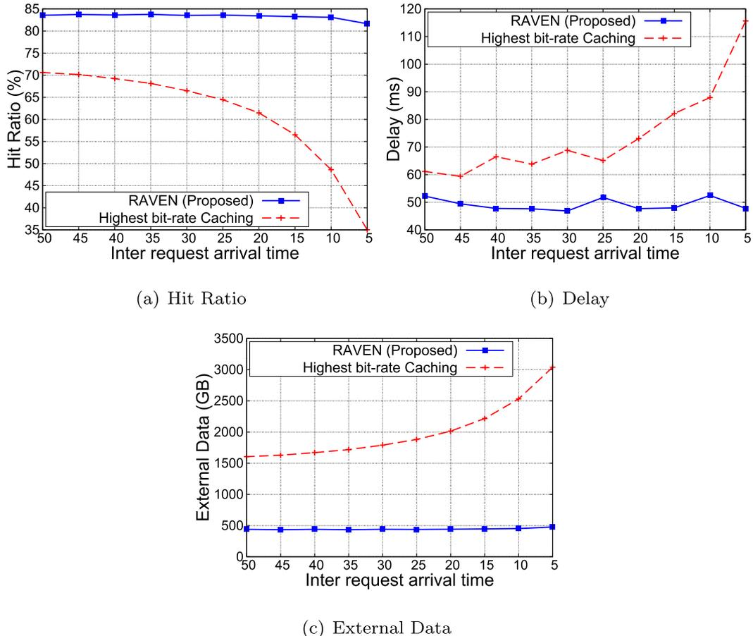
**Fig. 3.** Change in hit ratio, delay, and external data on varying the inter request arrival rate ( $\lambda$ ).
